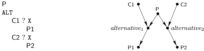
Fig. 1. A dynamic precedence graph representing P : the output mode of P is ALT and the input mode of alternative_1 and alternative_2 is PAR .
